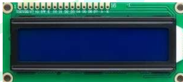
Gambar 2. 12 Liquid Crystal Display Sumber: https://www.thingbits.net (2020)
