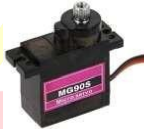
Gambar 2. 2 Motor Servo MG90S Sumber : m.media-amazon.com/ (2019)
